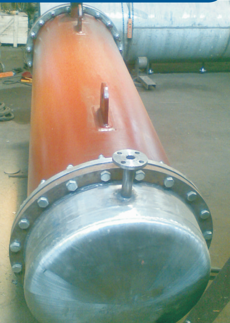
➡ 100 Sq. metre M S Shell - SS Tube type condenser
